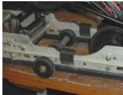
Two sets of idler wheels were added to reduce friction related noise and track slap.
