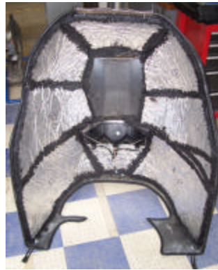
Insulation was installed and the seams were coated with quiet coat to prevent water absorption.
