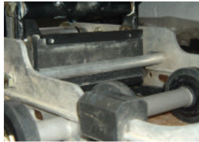
A rebound damper was added to reduce the metal-on-metal contact noise between the suspension and the cross-piece.
