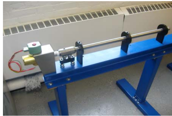
Fig5. Barrel, supports, flange and solenoid valve.
