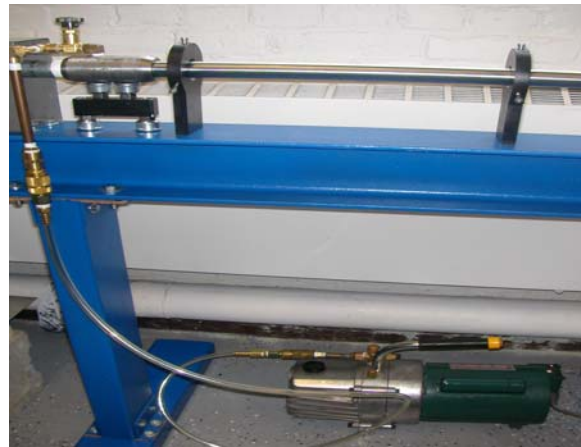
Fig8. Vacuum pump, tubing, and manual pressure valve.
