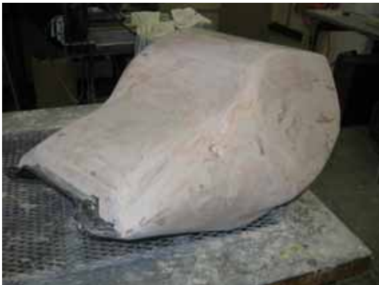
Figure 14. Final plug (unfinished surface)
