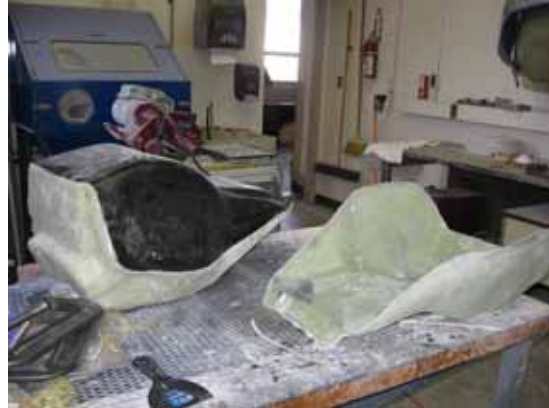
Figure 15. Finished plug with mold halves
