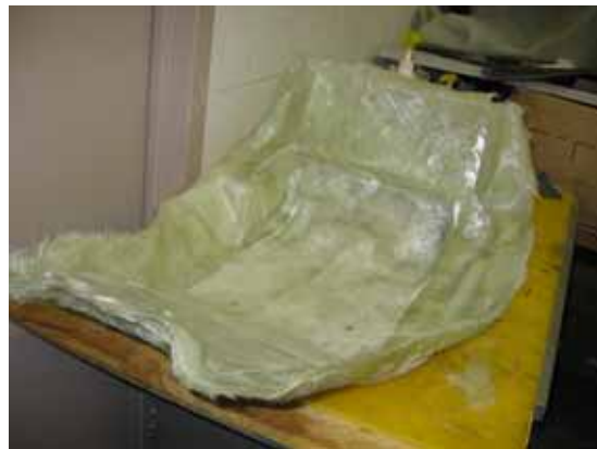
Figure 16. Lower mold half, laid up with fiber
