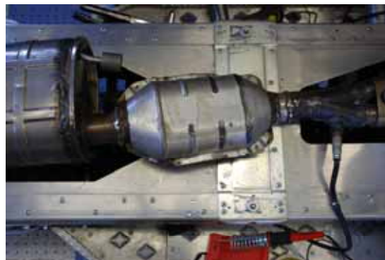
Figure 10. Catalytic Converter welded before muffler
