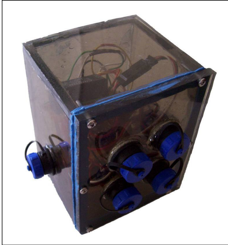
Figure 3.1.5 – Carrier board inside carrier board housing box
