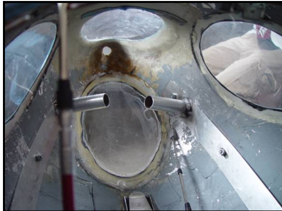
Figure 3.3.1 Newly mounted control mounting brackets
