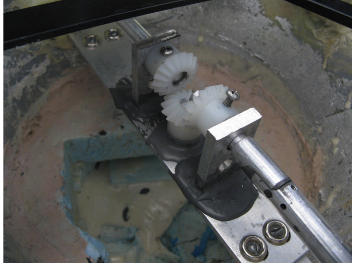
Figure 3.2.2 - 3-gear system used for opposite control surface movement
