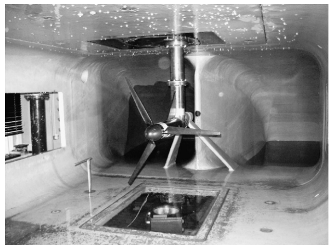
Fig. 2. Photograph of the assembled test rig in the cavitation tunnel.
