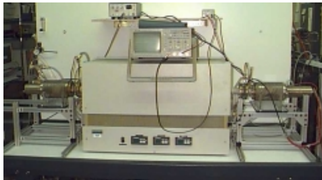
Figure 3: Furnace used for ultrasonic monitoring of oxidation of samples
