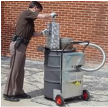
After the preliminary fire is started, drugs are injected into the fire with the EZ Feed system.
