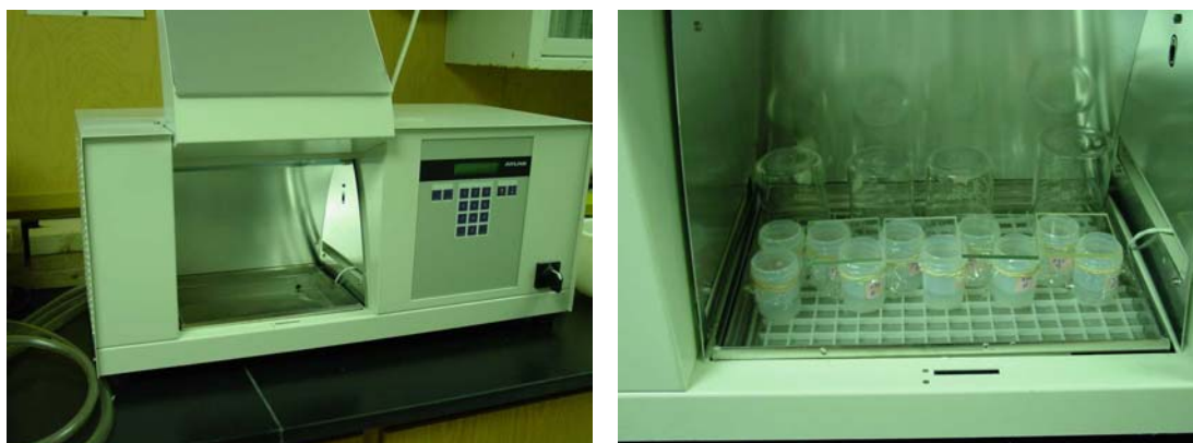
Fig. 1. Suntest tabletop xenon chamber used to expose samples to UV light, showing chamber (left) and Teflon cups (right).
