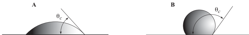
Fig. 1.1 Wettability of a surface, illustrated by the angle that a small, liquid drop makes with that surface. The angle is always measured inside the droplet. The more wettable the surface by the liquid, the smaller the contact angle, \theta_c , so that the surface in A is more wettable by the respective liquid than the surface in B .
