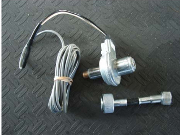
Figure 1: speedometer cable to voltage converter
