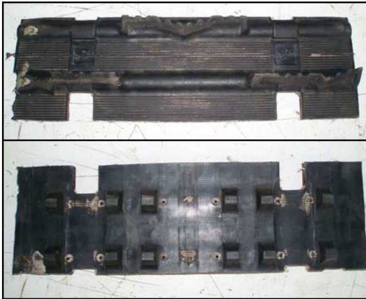
Figure 4 Old Arctic Cat Snowmobile Track with metal track- slider interface clip removed.
