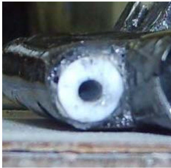
Figure 17 Deformation of Teflon bearings
