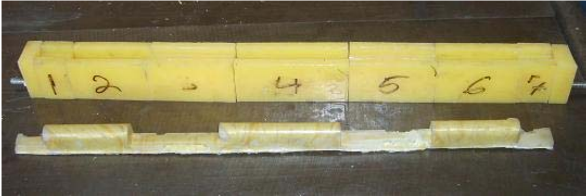
Figure 9 - Side mold and test piece constructed from mold
